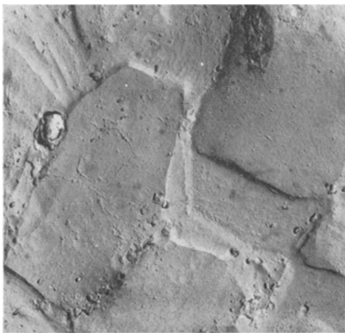
Figure 8 Carbon replica, showing the preferentially etched zones at tensile boundaries. Tensile axis approximately vertical. \times 9700 .
